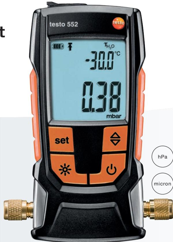
The testo 552 is a digital vacuum measuring instrument for the evacuation of refrigeration systems and heat pumps. It measures even the smallest absolute pressures and provides highly precise information on the status of the dehumidification of a system (removal of foreign substances, incl. oils or foreign gases).
